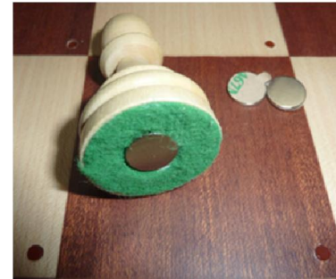
fix the neodym magnets with hot-glue
