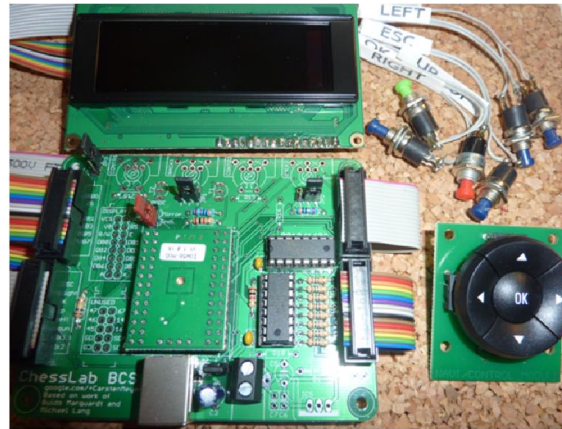
Assembly for version 1 with power supplied by USB solely
